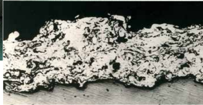
Fig. 3-3. Section through zinc sprayed coating.
