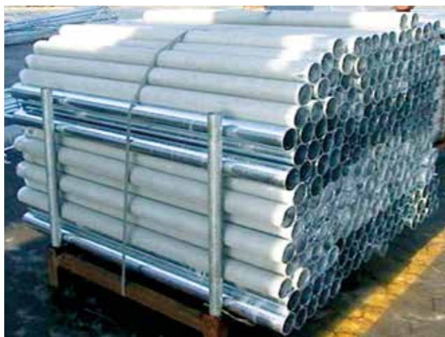
Fig. 5-7. Hot-dip galvanized tubes with different silicon content. Some of the tubes consists of aluminium-killed steel and have a shiny coating, while others consist of silicon-killed steel which gives a dull, grey coating.
