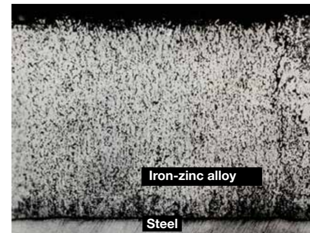
Fig 5-3. Cross-section through zinc coating on a steel in the Sandelin range, with 0.06% Si. Galvanizing carried out at 460 °C.
