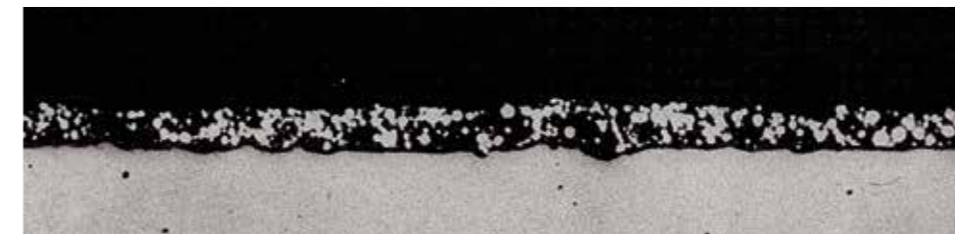
Fig. 3-4. Section through zinc-rich paint coating.
