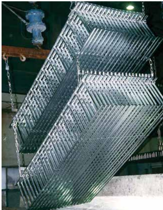
Fig. 7-1. Galvanizing of cable trays. Tilting the goods improves the run off of excess zinc when leaving the bath.
