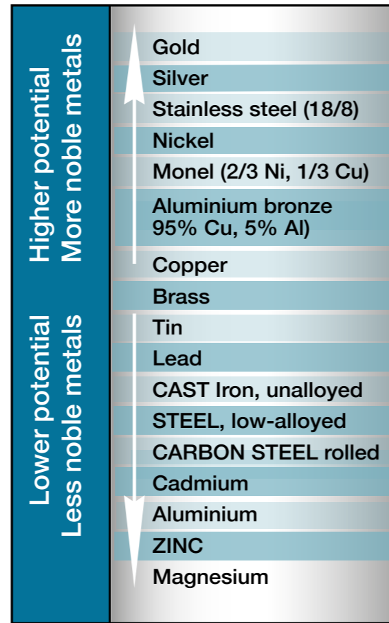
Fig. 10-10. Electrochemical potential scale in sea water at + 25 °C.
